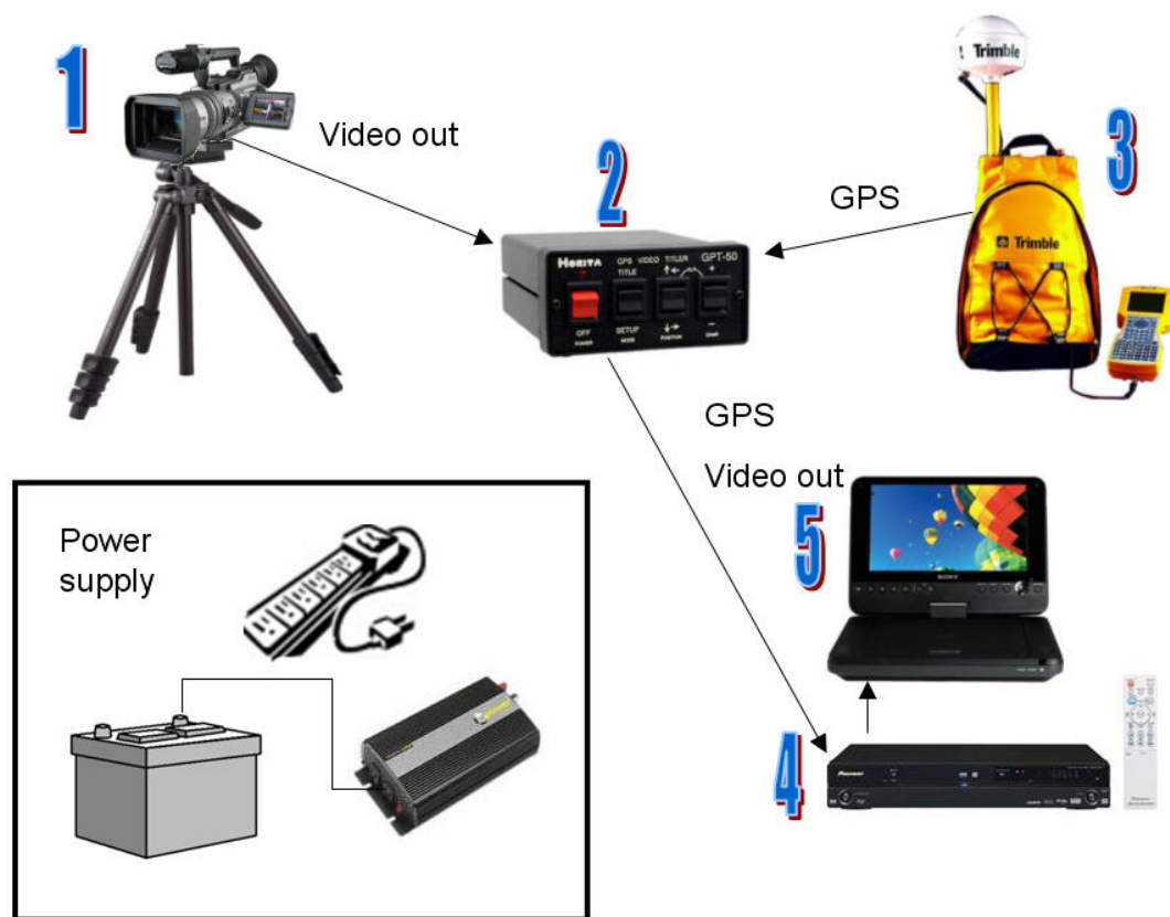
Figure 1: Shoreline video setup. 1) Digital video camera, 2) GPS stamper unit, 3) GPS data logger and receiver, 4) Digital video recorder, 5) Digital video player
