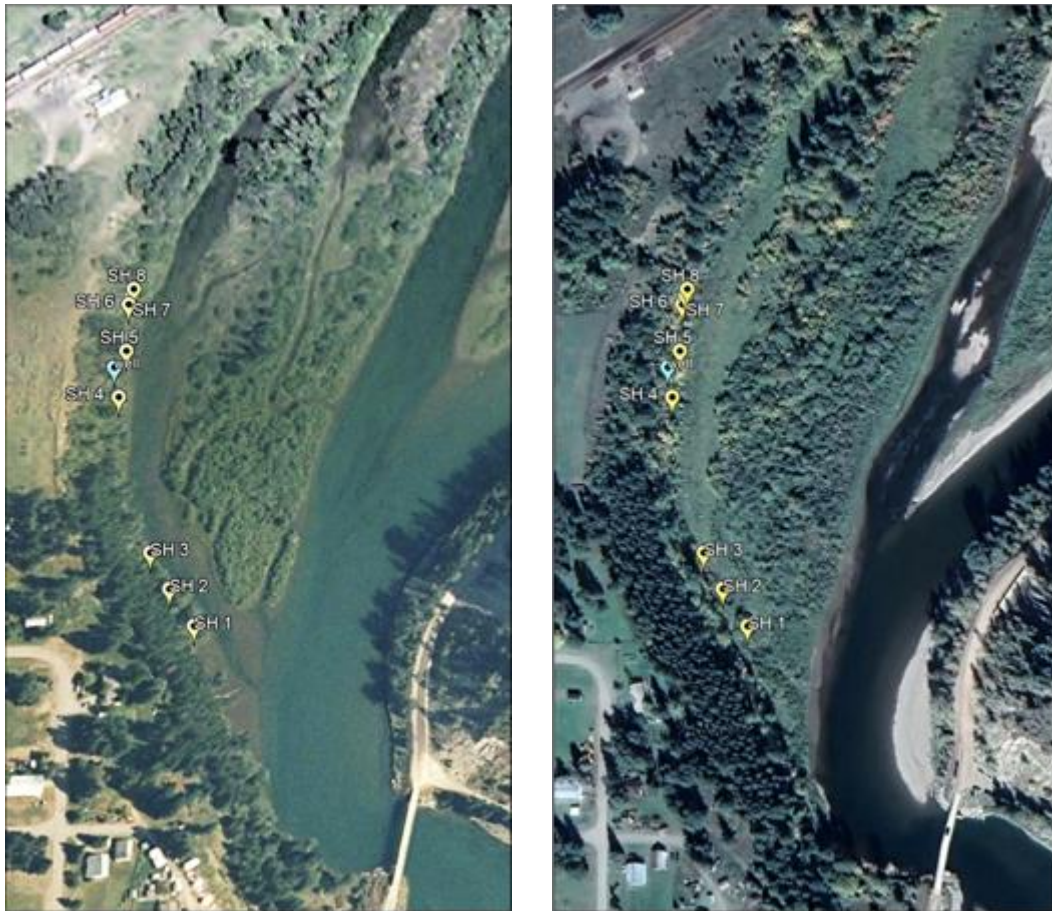
Figure 3: The aquifer recharge inlets along a back channel of the Elk River, below the steep bank at Elko, BC.
