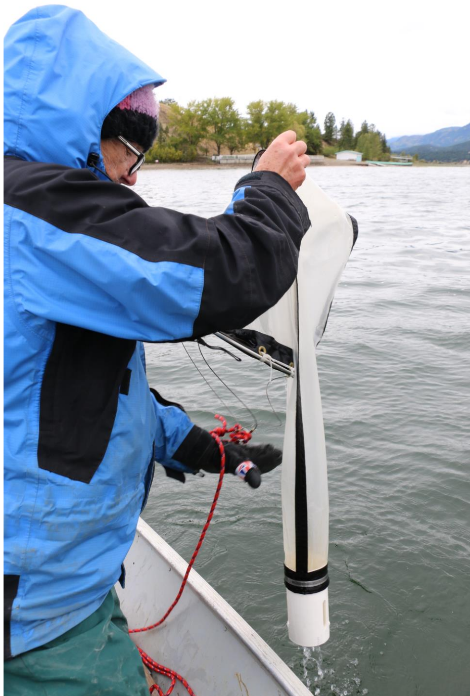
Figure 1. Plankton net used for a vertical plankton tow to test for invasive mussel veligers in the water column.
