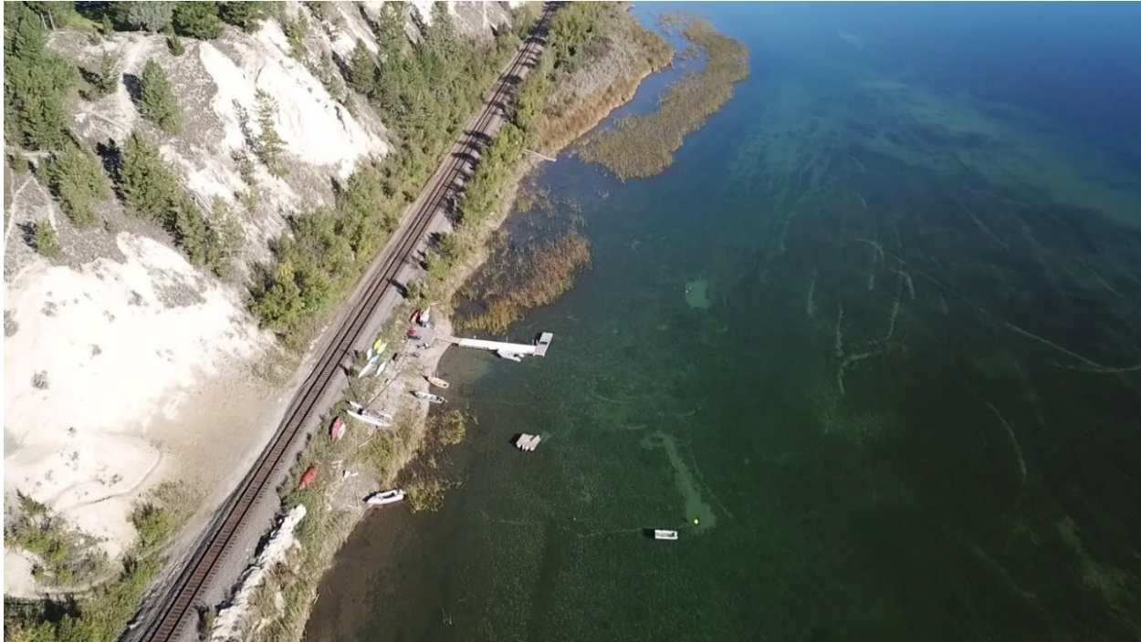
Figure 11: Erosion and aquatic vegetation disturbance caused by mooring buoy anchor scour and boat propeller drag observed along the west shoreline of Columbia Lake in Segment 6.
