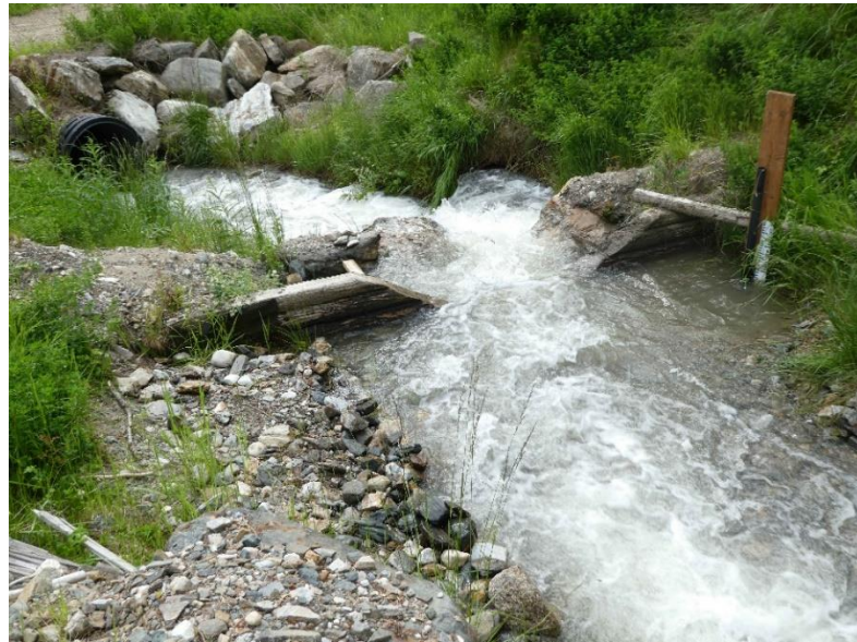
b) Gar station – staff gauge and weir
